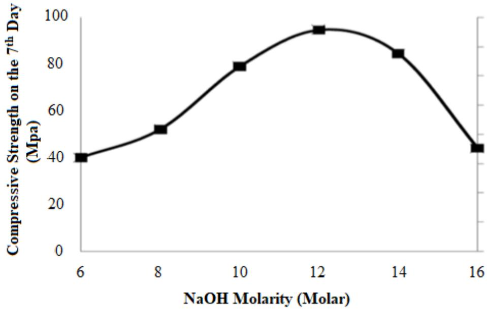
Fig. 4 Effect of Molarity on the Compressive Strength of Concrete<sup>16</sup>
