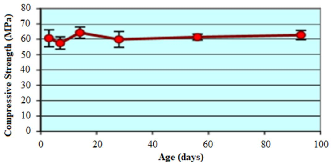
Fig. 10 Compressive Strength of Geopolymer Concrete at different ages<sup>25</sup>
