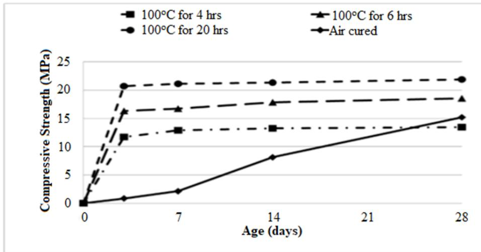
Fig. 8 Compressive Strength of Geopolymer mortar cured at 100°C for 4, 6 and 20 hours<sup>24</sup>
