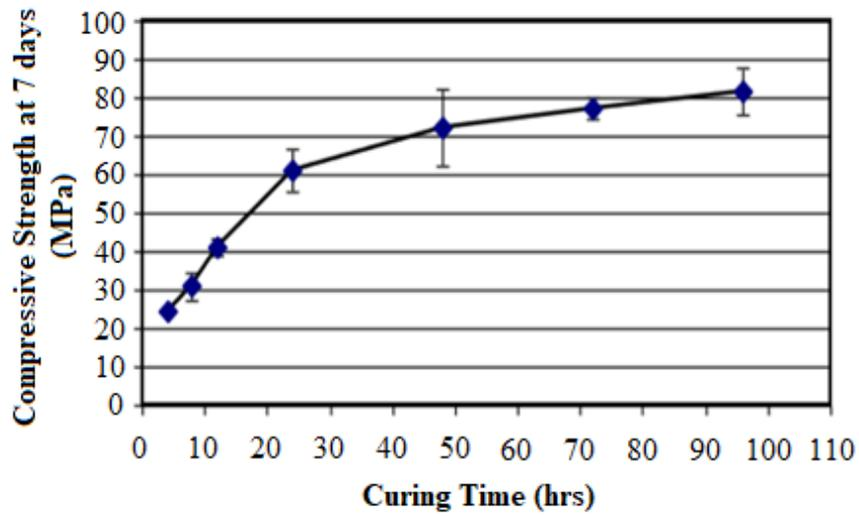
Fig. 6 Effect of curing time on the Compressive Strength of Concrete<sup>14</sup>
