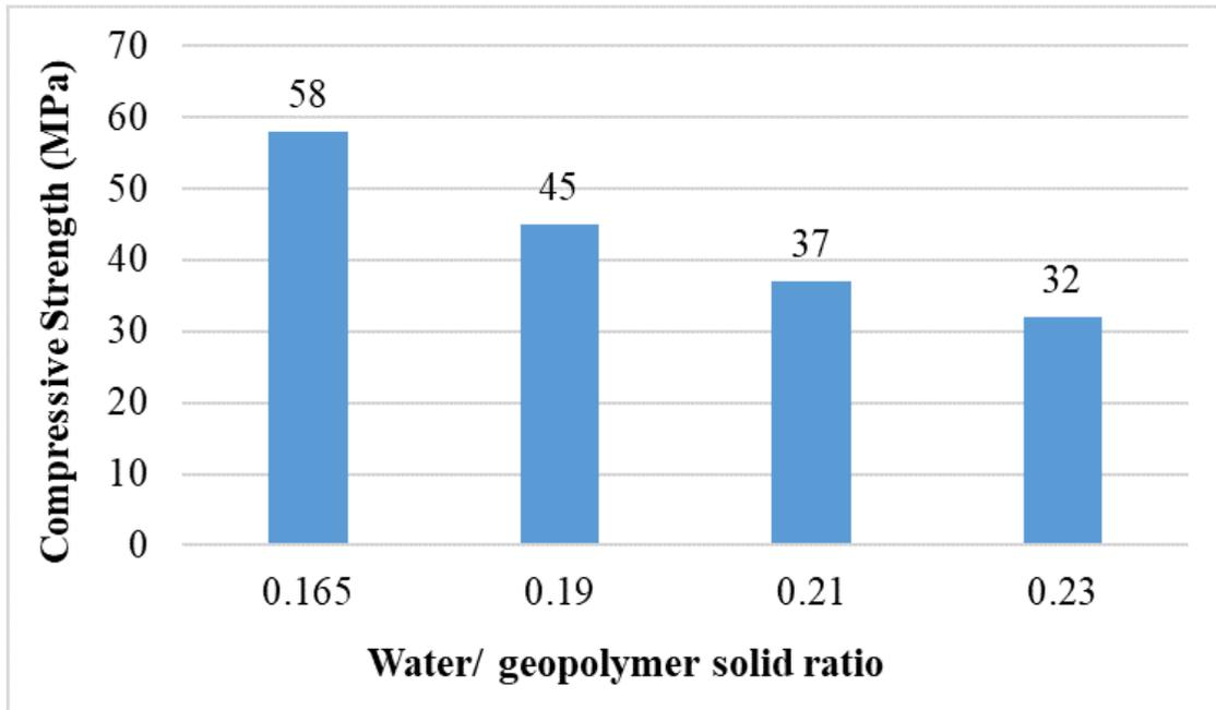
Fig. 2 Effect of water/ Geopolymer solid ratio on the Compressive Strength<sup>5</sup>
