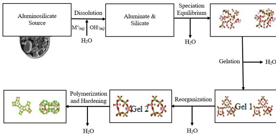
Fig. 1 Geopolymer reaction mechanism model<sup>9</sup>
