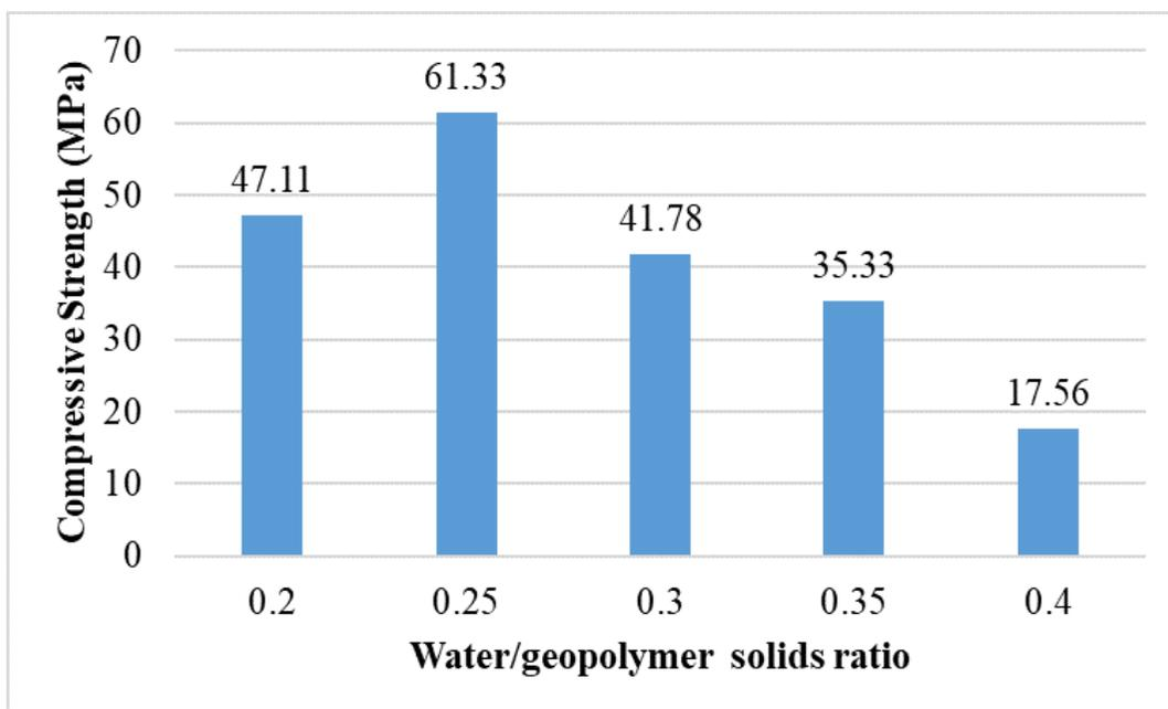
Fig. 3 Effect of Water/ Solids ratio on the Compressive Strength<sup>15</sup>
