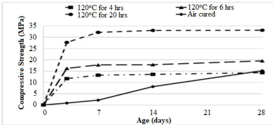
Fig. 9 Compressive Strength of Geopolymer mortar cured at 120°C for 4, 6 and 20 hours<sup>24</sup>
