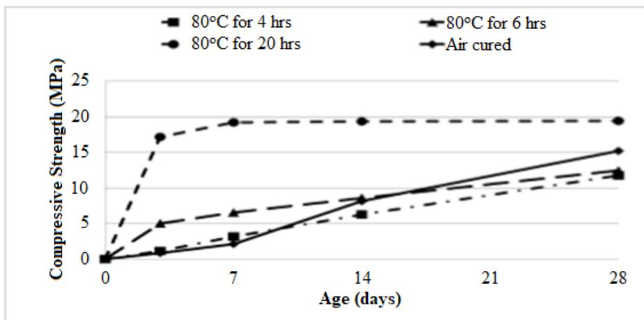
Fig. 7 Compressive Strength of Geopolymer mortar cured at 80°C for 4, 6 and 20 hours<sup>24</sup>
