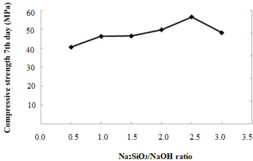
Fig. 5 Effect of Na<sub>2</sub>SiO<sub>3</sub>/ NaOH on the Strength of Concrete<sup>16</sup>
