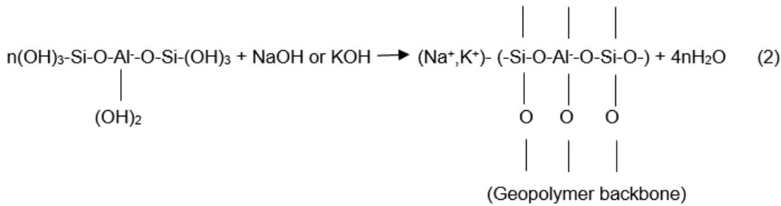
It is evident from equation (2) that water is expelled during the chemical reaction in the formation of Geopolymers. The water thus released benefits the performance of Geopolymer as it leaves behind discontinuous nanopores during curing and further drying periods.
