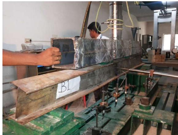
Fig.7(a) Failure pattern of 100 mm Beam
