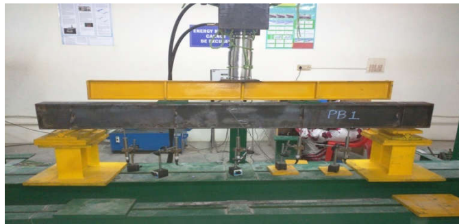
Fig. 4. Experimental set-up for Test Beams
