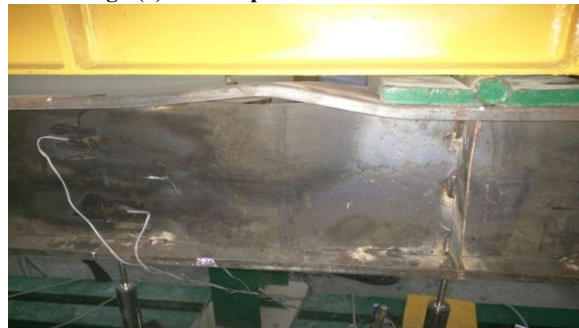
Fig.7 (b) Failure pattern of 200 mm Beam
