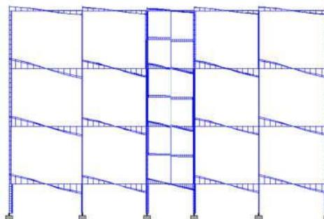
Fig5. Shear force diagram
