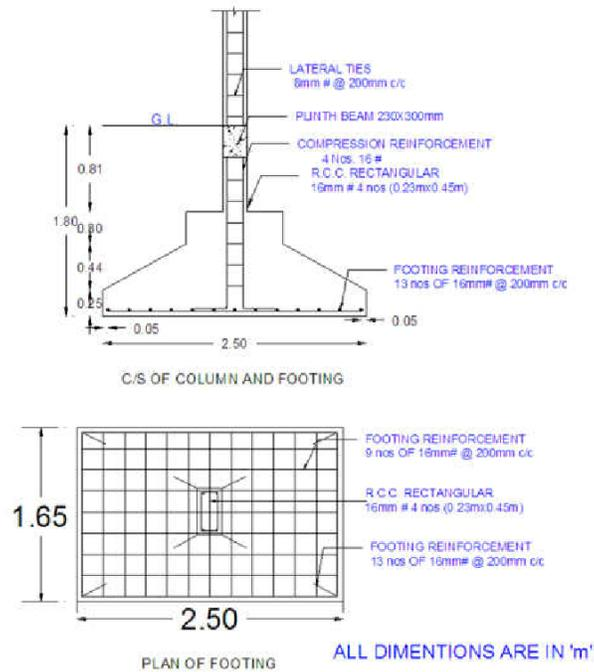
Fig10. Column and footing reinforcement.
