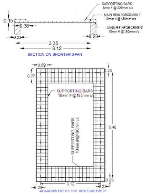
Fig7. Two way slab reinforcement
