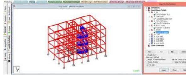
Fig 7 Load due to staircase
