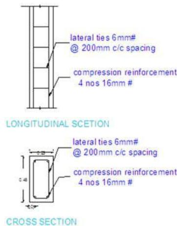
Fig 9 .Column reinforcement
