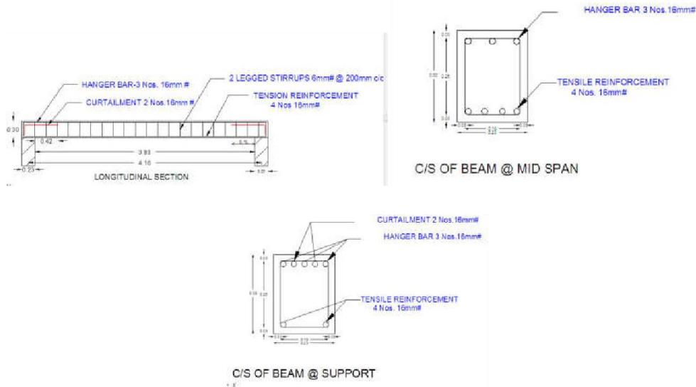
Fig 8. Beam reinforcement
