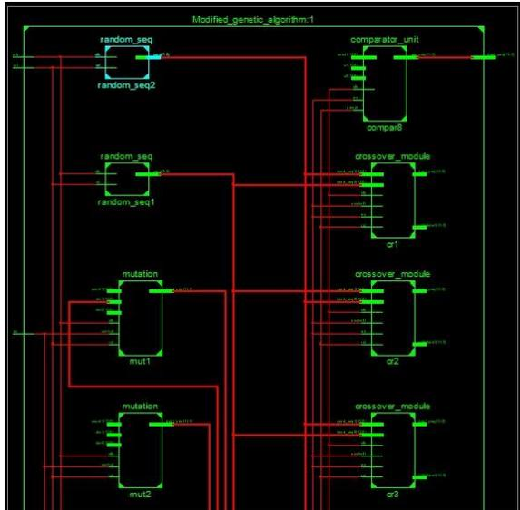
Fig.2. RTL Schematic of the MGA.
