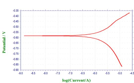
**Figure 3: Potentiodynamic polarization test in Al2024/0% flyash in 0.035%KCl**
