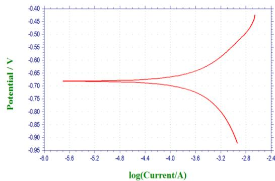
Figure 12: Potentiodynamic polarization test in Al2024/2% flyash in 3.5%KCl
