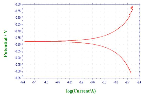
Figure 14: Potentiodynamic polarization test in Al2024/6% flyash in 3.5%KCl
