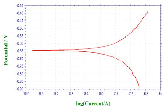
**Figure 8: Potentiodynamic polarization test in Al2024/2% flyash in 0.35%KCl**
