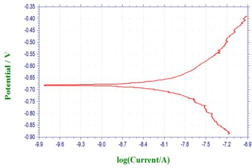
Figure 9: Potentiodynamic polarization test in Al2024/4% flyash in 0.35%KCl
