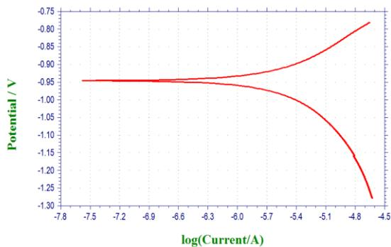
**Figure 5: Potentiodynamic polarization test in Al2024/4% flyash in 0.035%KCl**
