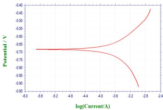
Figure 11: Potentiodynamic polarization test in Al2024/0% flyash in 3.5%KCl
