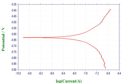
**Figure 7: Potentiodynamic polarization test in Al2024/0% flyash in 0.35%KCl**
