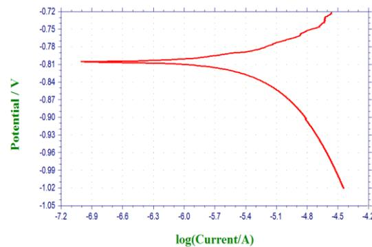
**Figure 6: Potentiodynamic polarization test in Al2024/6% flyash in 0.035%KCl**
