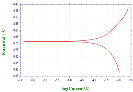
Figure 13: Potentiodynamic polarization test in Al2024/4% flyash in 3.5%KCl
