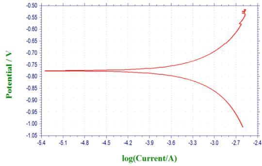
Figure 10: Potentiodynamic polarization test in Al2024/6% flyash in 0.35%KCl
