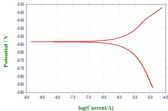
**Figure 4: Potentiodynamic polarization test in Al2024/2% flyash in 0.035%KCl**
