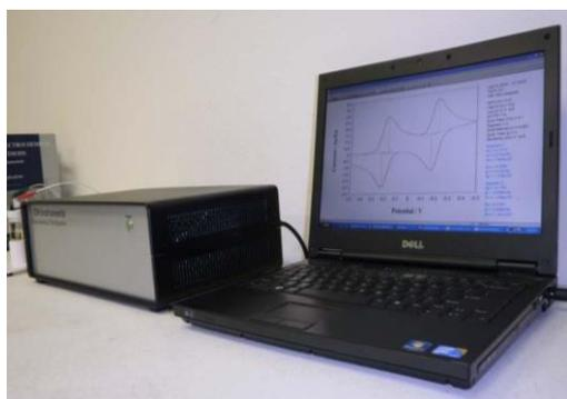
Figure 1: Electrochemical workstation
